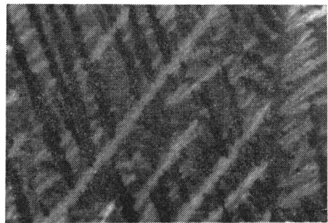
Fig.5 Micrograph of polyethylene spherulites grown near the edge of the same sample as shown in Fig.3.
